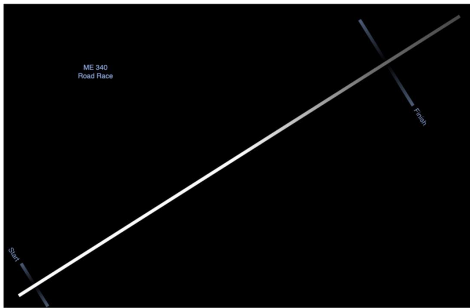
Figure 1. Course that our robot is to navigate [2]. The key aspect to this course is speed. However, one aspect that is challenging is that the line gets dimmer the further the robot travel and the robot has to autonomously stop at the end of the line.
